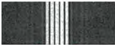
For d = 4a , every fourth interference maximum at the sides ( m_i = \pm 4, \pm 8, \dots ) is missing.
